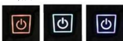
To turn off the heating of the vest, it is necessary to press the switch for 3–5 seconds.
